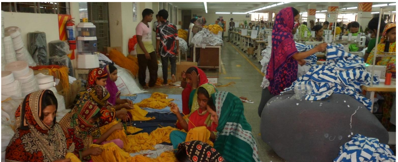
Image 8: Blocked escape routes
